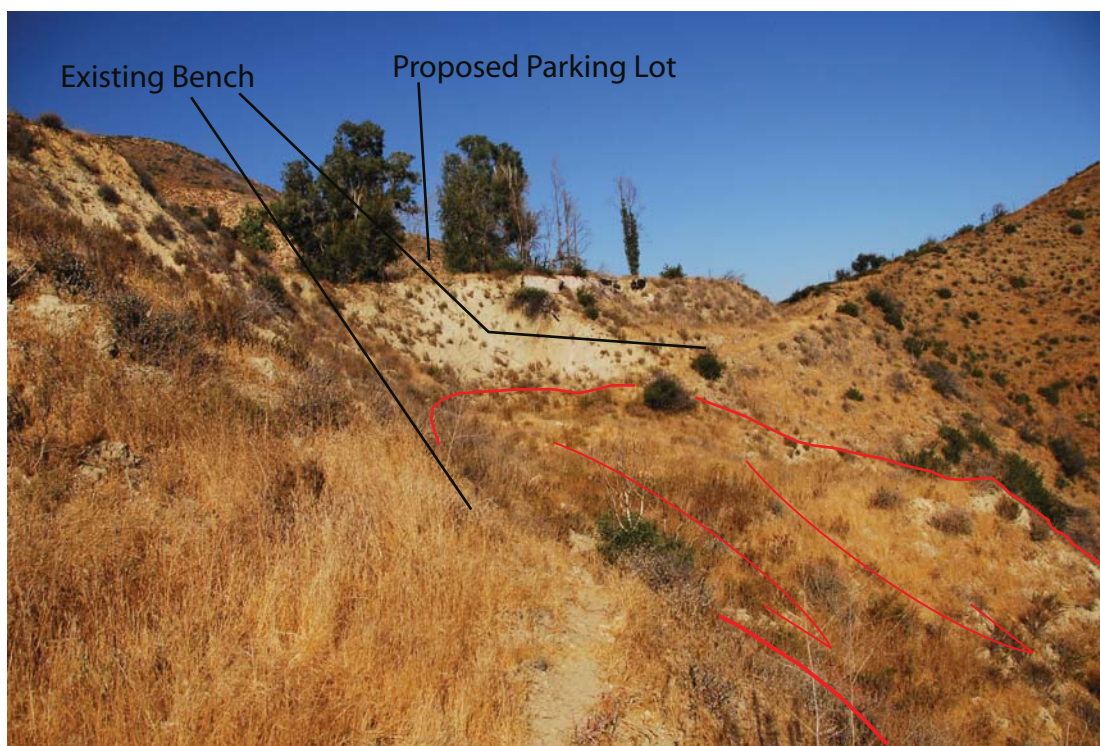
Photo 14 - View looking east across landslide south of proposed parking area, showing headscarp and displacement of existing trail.
